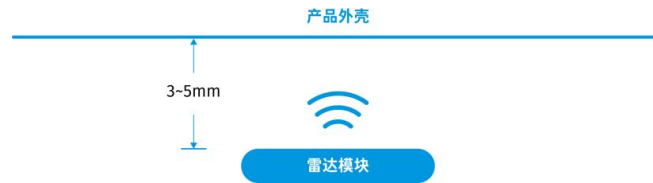
Figure 4 Distance between antenna surface and product housing
