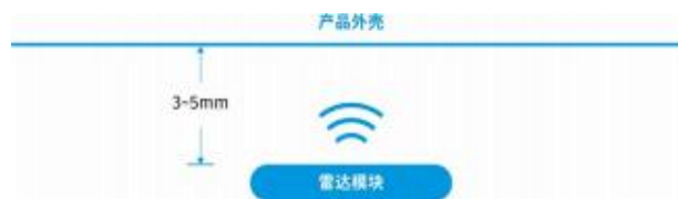
Figure 4 Distance between antenna surface and product housing
